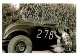
Racing at El Mirage meant removing the headlights, bumpers, windshield, and fenders. Bernie began with a stock Flathead V-8, so every part removed helped him go faster. But all these parts were carefully stored in the back of his garage.
